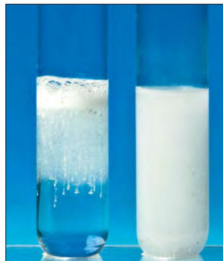
Figure 8.12 Magnesium reacting with a strong acid (hydrochloric acid, left) and a weak acid (ethanoic acid, right). The more violent reaction with the strong acid causes larger hydrogen bubbles, which keeps the magnesium at the surface of the fluid. The much smaller bubbles caused by the weaker acid reaction spread through the acid, making it appear milky.
